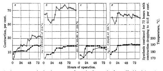
Fig. 1.—Apparent contraction O and temperature of operation  $\bullet$  versus time for test 73 with cobalt catalyst 108 B at atmospheric pressure. Catalyst was reduced in hydrogen at 360° and carbided with carbon monoxide at 200° for twenty-four hours prior to testing.
